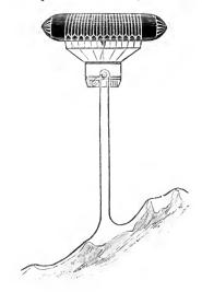
over a pulley situated in the car of the balloon. The pulley is rotated by an electro-motor in the car and thus draws the balloon along in the direction of the rope.
